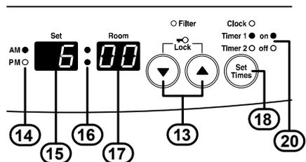
The factory default Timer 1 'On' time is AM 06:00. Press the Up or Down buttons (13) to adjust the Timer 1 'On' time.
