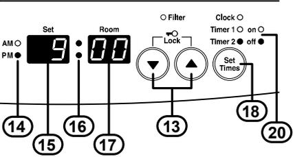
The factory default Timer 2 'Off' time is AM 09:00. Press the Up or Down buttons (13) to adjust the Timer 2 'Off' time.
