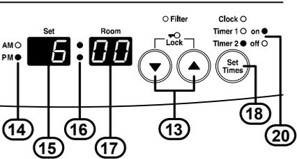
The factory default Timer 2 'On' time is AM 06:00. Press the Up or Down buttons (13) to adjust the Timer 2 'On' time.
