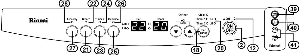
**NOTE** **Timer 1 and Timer 2 may be operated together or individually. The heater will continue to operate under control of the timers until timer operation is cancelled.**
