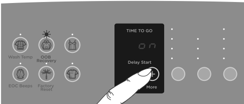
Fig.28 Changing the out of balance recovery routine
