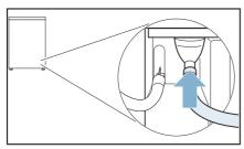
Secure the other end of the drain hose in place using the remaining accessories (depending on the connection type).
