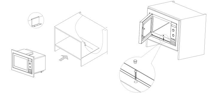
• Slide the appliance into the housing unit, and pull the cable with the plug\* through the back of the unit.
