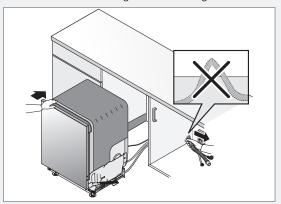
7 Make any final adjustments to the front feet (the dishwasher may lean no more than 5 mm) and tighten the lock nuts.
